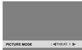
\* If neither the ◀ or ▶ button is pressed within 5 seconds, the current selection is set and the previous screen reappears.
