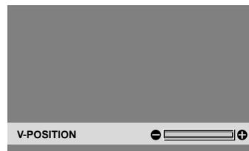
\* If neither the ◀ or ▶ button is pressed within 5 seconds, the current setting is set and the previous screen reappears.
